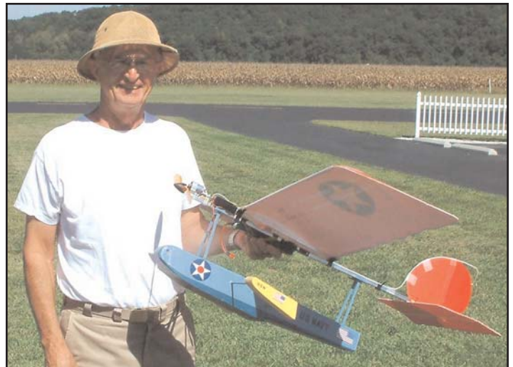
George Cooper goes electric with his GWS Slow Stick. It has a GWS 350 motor with a 6.6/1 gearbox and a flying boat hull. We can't wait to see a water takeoff!
