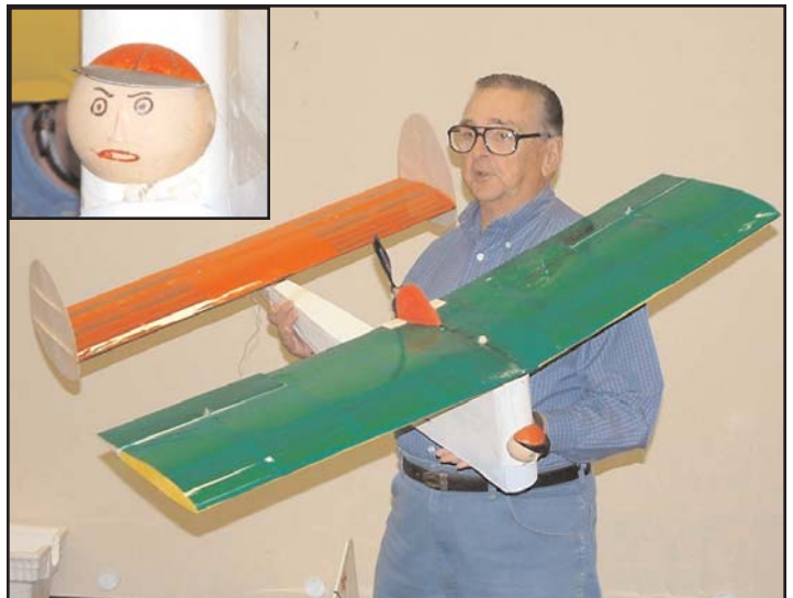
Don Fitch prompted an extensive discussion about the design concepts he used when scratch-building his "E-Boy". It has an AXI 2208/34 brushless electric motor and weighs 25 ounces. The inset picture is his pilot, on the front of the pylon.
