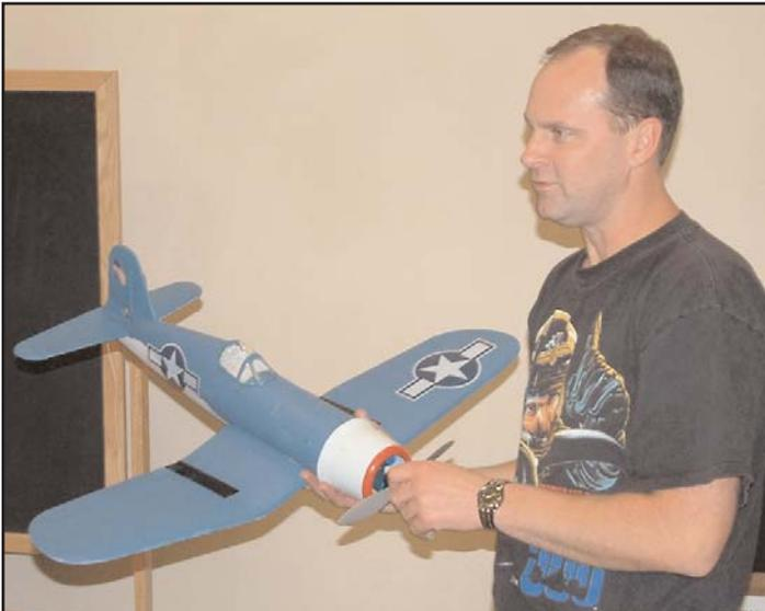
*Greg Bohrer discusses a GWS Corsair he helped Harold Mantz build. It's foam construction and has a brushless motor. Harold reinforced critical areas with fiberglass and carbon fiber and finished it with indoor latex wall paints. It flies well, but is a bit fast for Harold's tastes.*
