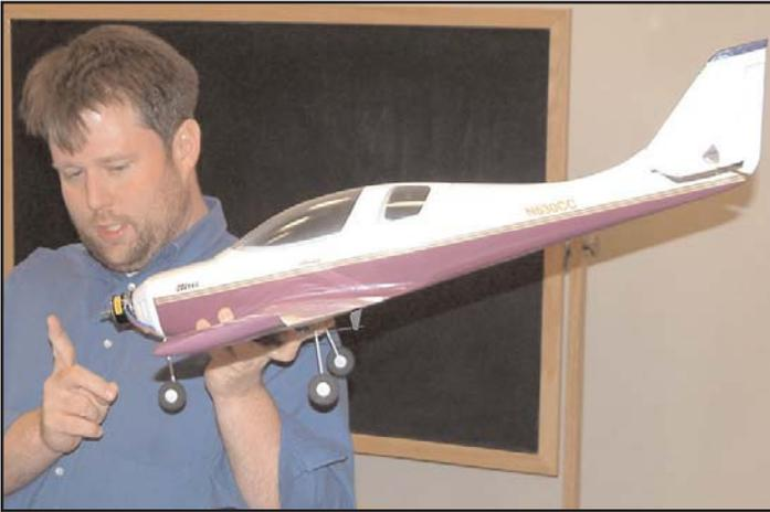
*Duane Youngman discusses his new Great Planes Electrify Lancair ES EP ARF. It has a fiberglass fuselage and built-up balsa wing. He modified it by replacing the supplied geared speed 400 motor with an E-Flite 480 brushless unit. Weight is 26 ounces. A very nice ARF for \$94.95!*
