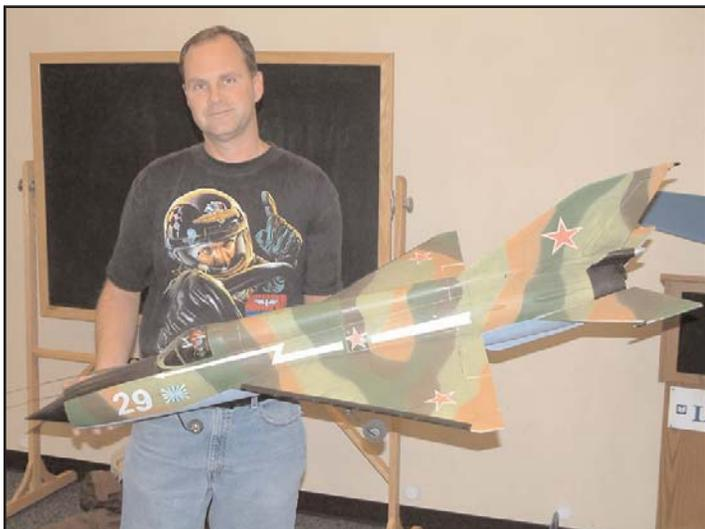
*Greg Bohrer discussed problems encountered and construction techniques he used scratch-building this Depron foam Mig 21. It has a 70 MM ducted fan and weighs 70 ounces. It flies well, but isn't as fast as he had hoped it would be. Greg posted a "build log" on RC Groups web site at:*
