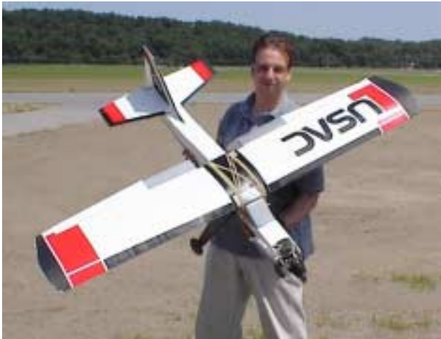
Kevin Gianino shows his U. S. Aircore Nighthawk. It's powered by a Thunder Tiger .46 Pro engine and has a Futaba six-channel radio. He says its a little harder to build than a balsa plane would be, but much more durable.
