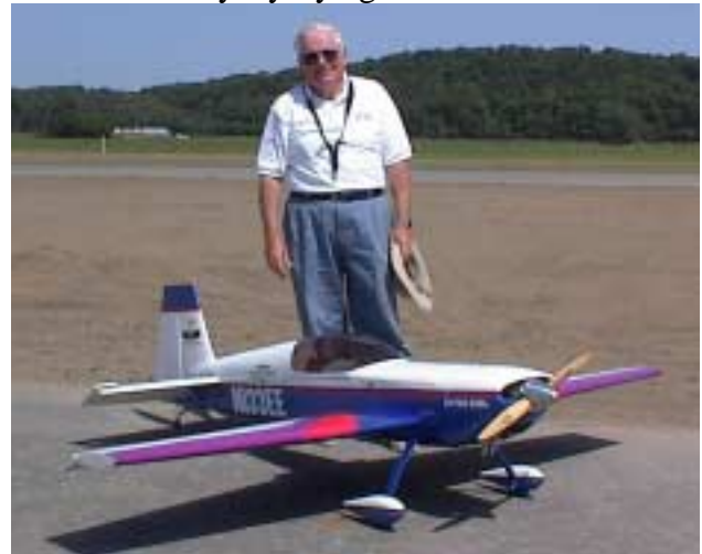
Bob Underwood with his Hanger 9 ARF Extra 330L. Power is by a Zenoah G-62 and he guides it with a JR ten-channel radio. He says its well-built and flies very nicely. He feels that the computer radio is very easy to program.. It weighs 24 pounds, even after Bob did some lightening of the structure.
