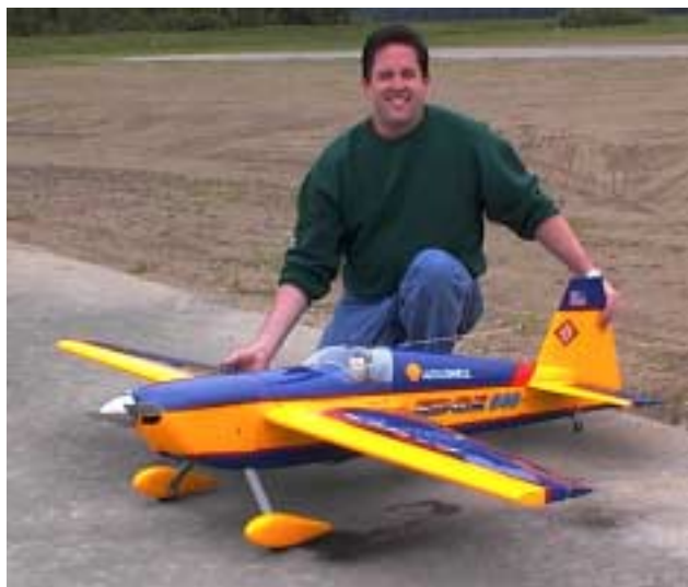
Craig Finks immediately after flying his Hanger 9 Edge 540 ARF for the first time. The Saito 1.80 four-stroke hauls it around beautifully at half-throttle!
