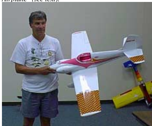
Bob Fiely shows his Sig 450 Midget Mustang. The engine is a K&B quickee 40 rear exhaust type and the radio is Futaba four-channel. It hasn't been flown to date.
