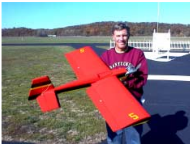
Bob Fiely shows his Great Planes Dazzler. He's recovered it three times and flown it hundreds of times. It has an O.S. .46 FX up front.
