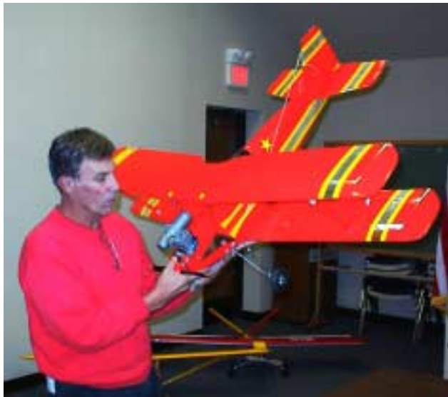
Bob Fiely shows and discusses his new Great Planes Aeromaster. He has modified it and it's powered by a Super Tigre .61 ringed engine. It weighs 7 pounds, 5 ounces.
