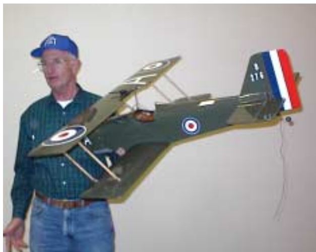
George Cooper kit-bashed a Sig Smith Mini-Plane to build this SE-5A. It's powered by an O.S. .46 FX and is covered with Monokote. He hasn't flown it yet.
