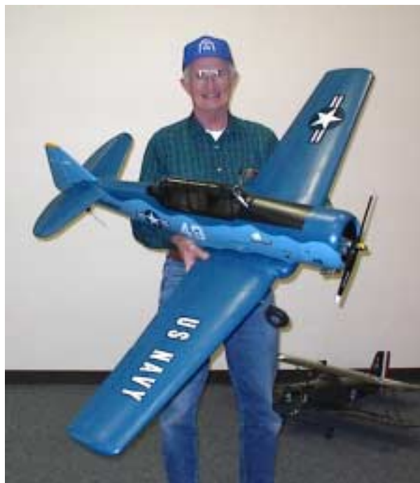
George Cooper brought his Top Flite AT-6. It's powered with a Saito .91 four-stroke and has Robart pneumatic retracts. He finished with latex house paint and water-based polyurethane clear. It hadn't been flown at meeting time.
