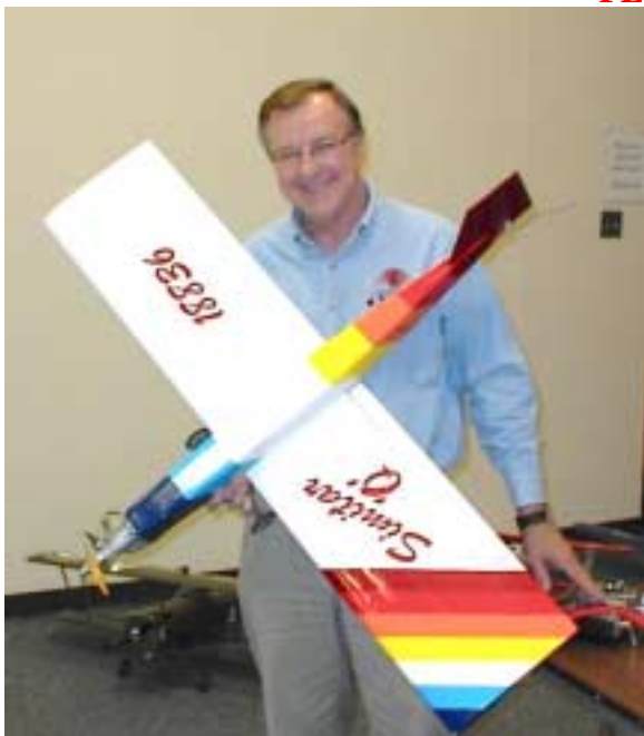
Paul Geders built this Bill Evans-designed Simitar "Q" some years ago. It's powered by a Rossi .40 S/N 002 with a "zero boost" muffler! Look Ma, no elevator and it flies great!
