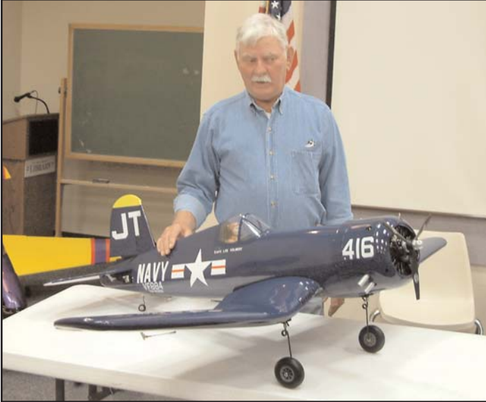
Lee Volmert shows his Super Tigre .75-powered Hanger 9 F4U Corsair ARF. It came in ten pieces, all of which fit perfectly. It's all wood construction covered with Ultracote. The retractable gear is very troublesome, but Lee's working on it.
