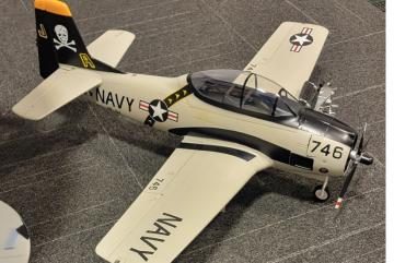
This has a 750KV brushless outrunner motor driving a 3-blade propeller controlled by a 40-amp ESC. It has retracts, and seven 9 g servos. It runs off a 4S Li-Po.
