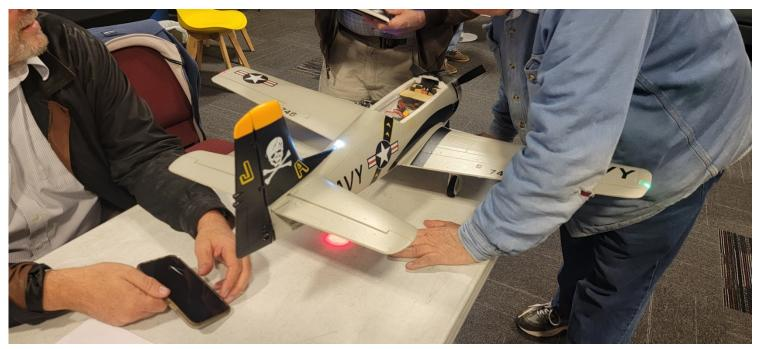
Next was Wayne Nenninger's FMS Ranger. This model has a majestic 1800mm wingspan (70.9 inch) and flies on 4S power. It turns a 12 x 7.5 propeller via a 750kv motor and 45-amp ESC. It is float capable and has STOL characteristics with functional flaps and oversized wheels making all terrain flights easier.
